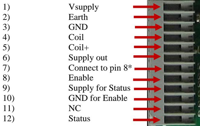
\*: This pin 7 has to be connected to pin 8 to operate the solenoid; this is done directly on the female connector
