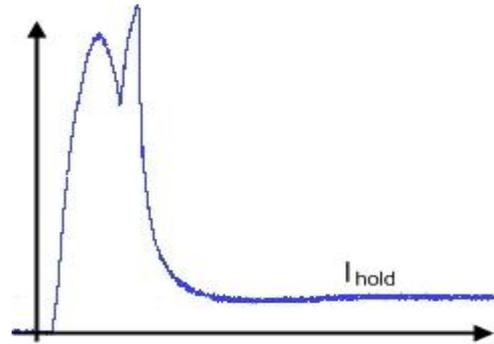
Figure 1: Typical current pattern using the ADRV1012K
