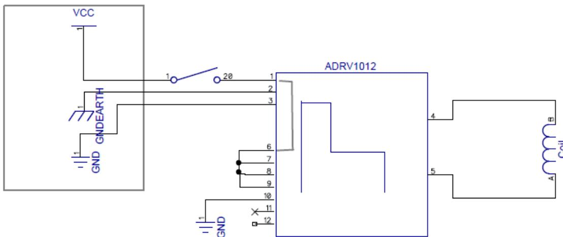
To use the device in two wire mode (ON/OFF by switching on or off the power supply) connect as described on the schematics above. This mode is only recommended for slow operation as there is a 150ms delay to start the ADRV1012K driver.
