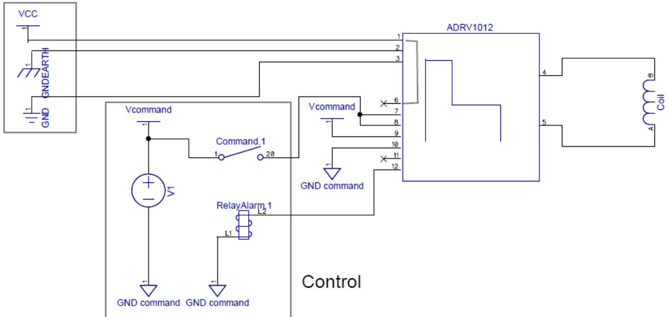
The driver can be driven by an external source such as a PLC or a relay. Switching the Enable (Pin 8) will switch the solenoid on or off. The output can be connected to an alarm. In case if the Enable is activated using the same power supply, Supply for Status (Pin 9) can be connected to Power supply out (Pin 6).
