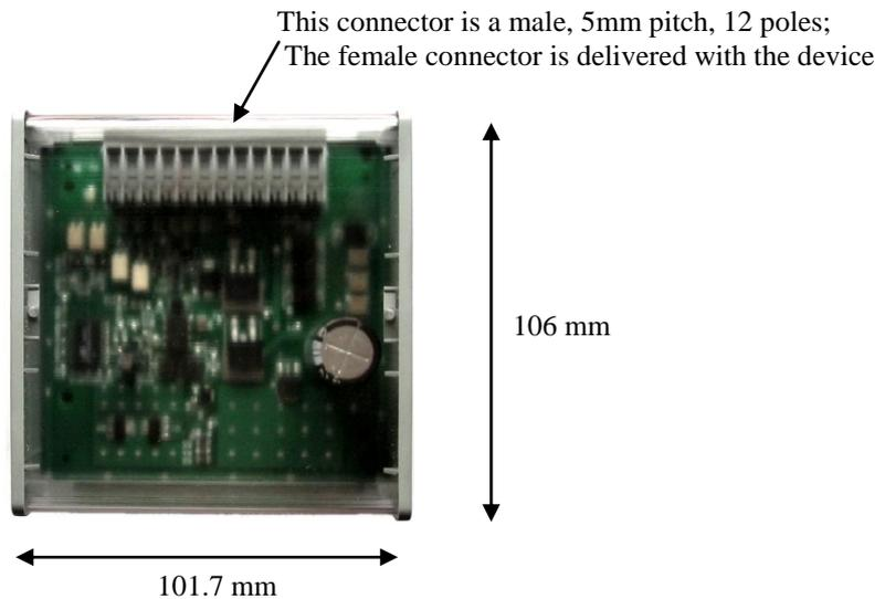
The device can be directly put on a horizontal plane, or on a DIN rail (there are fixing feet for mounting on DIN 35 rails on the bottom of the enclosure)
